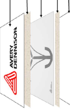
wet RFID inlay die-cut inlays with adhesive on liner
